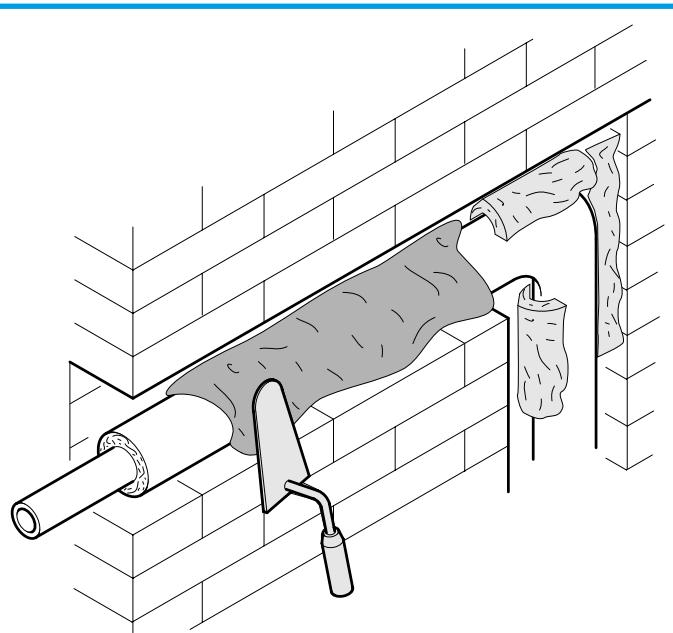
*Figure 1 – Inside wall pipe laying*
