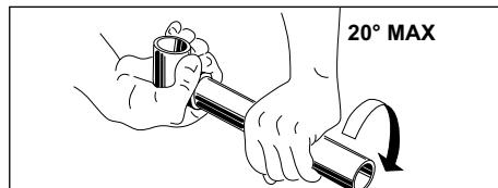
Any alignment implying pipe or fitting rotation must be carried out during or immediately after insertion without exceeding 20°.
