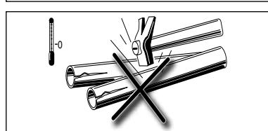
At temperatures lower than 0°, prevent impacts (especially against pipe ends), excessive loads, crushing or bending. Do not use pipes that are broken, cracked or dented.
