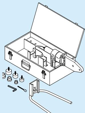
**1** Welder 800 W - 230V a.c. - 50 Hz, model **00NSBEP** supplied in a special case, complete with diam. 20-25-32 pairs of dies. The welder is equipped with an automatic thermostat to keep the die temperature constant at  $260 \pm 10^\circ\text{C}$ .
