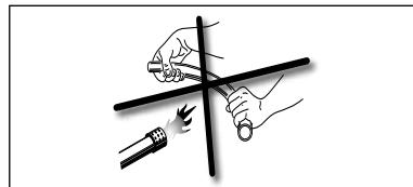
Do not use flames to work the pipes and obtain bends or crossovers, as being unable to control temperatures may lead to polypropylene molecular structure damage. Max 90° pipe bending angles can be obtained by cold bending, ensuring that the curvature radius is not smaller than 8 times the pipe diameter.
