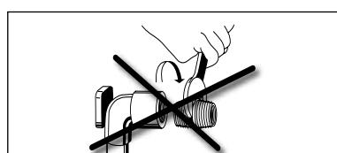
We recommend to avoid jointing by cast iron conical or non-calibrated threads as high tightening torques would break female brass unions. To ensure tightness, we recommend to interpose Teflon. The use of hemp packing in the right amount is also acceptable.
