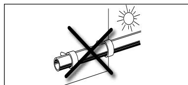
Always use the NIRON System under chase or wherever it is protected against weathering, to prevent damages mainly caused by short wave UV radiation combined with atmospheric oxygen. For this reason, pipes and fittings are supplied contained in suitable plastic bags or cardboard boxes.
