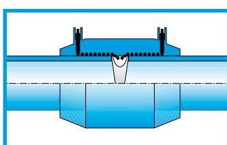
■ If the cut is not at right angles, there may be molten material dripping into the electric part and blocking the passage.
