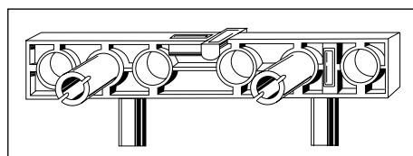
Use the specially designed templates to obtain correct alignment of the connectors in under chase installations.
