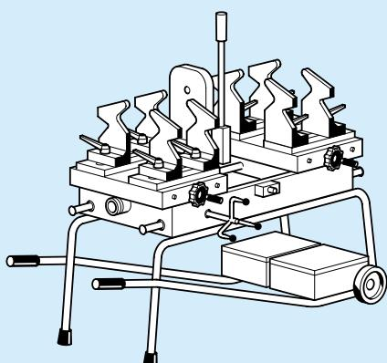
**2** Welder on wheels (see drawing) 1400 W - 230V a.c. - 50 Hz, model **00STL125** supplied on pallet and complete with case and diam. 25 to diam. 125 dies and pipe support.
