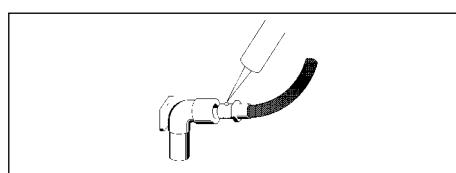
If liquid sealant is used to ensure tightness (art. NSF), remember to wait 1 hour at 20°C and 3 hours at -10°C before testing.
