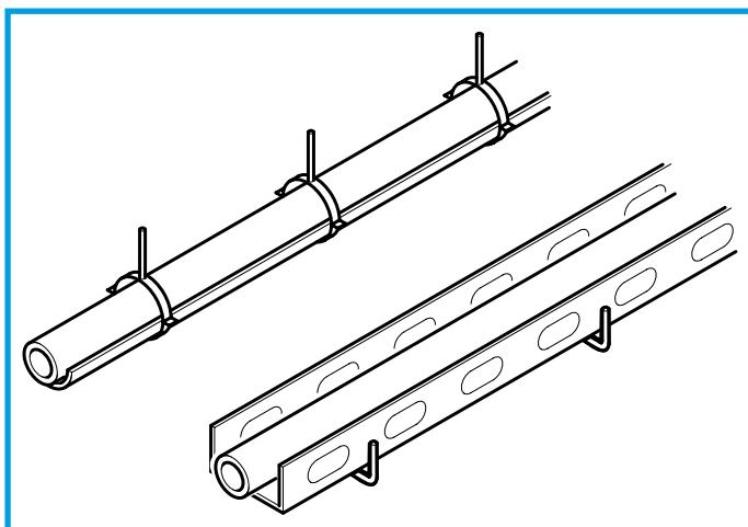
**Figure 2 – Installation on horizontal supports**
